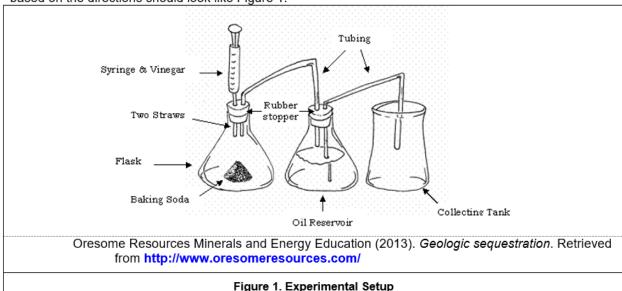
Remind the students to make sure the tubing is not kinked, and to hold the stoppers on the flasks so they do not pop off. Do not run the reaction without safety glasses.
