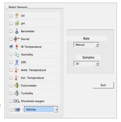
If you are using a DataHub brand external sensor attached to the Universal Adapter port, it will show up in the set up menu after you have attached it.
